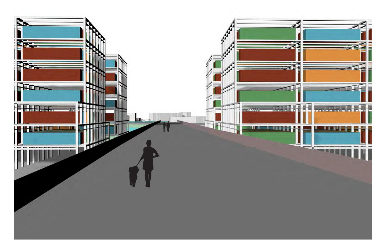
The existing yard holds up to 2,000 containers. The new vertical system doubles that with a 3,185-container capacity using just 20% of the land. Freight flow improves while freeing space for public use.
